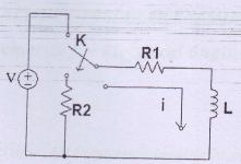
(B) In the network shown in fig., V1 = 3V,  $R1 = 10 \Omega$ ,  $R2 = 5 \Omega$ , L = 1/2H. The network attains a steady state at t = 0. The switch is then closed. Find particular solution of Va(t).
