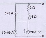
(B) Find Resistance 'R' and power by maximum power transfer theorem in the given circuit shown in below figure.
