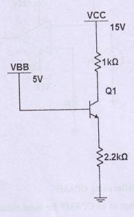
A. Calculate input impedance for following circuit if current gain is 100 for both transistors. (0
