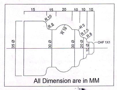
(B) Write a CNC Machining Center Program of given components.
