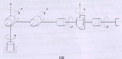
Q.2 Derive forward kinematics model for following 2D planar robot. Using this forward (10) kinematics model, derive inverse kinematics model to determine joint angles for given pose and position of end-effector.
